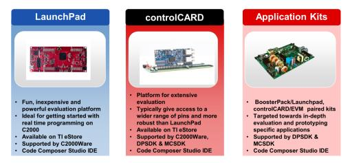
Fig. 1.1: Hardware - LaunchPads, controlCARDs or Application Kits
