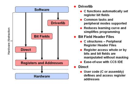
Fig. 2.2: DriverLib, Bit field and direct regiser access
