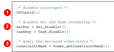
The next few steps analyze some of the current constraints on power savings. The returned constraintMask is checked (step 4) to see if the LPDS sleep state is allowed.
