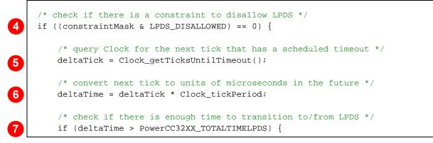
If there is sufficient time to transition in and out of LPDS, then the policy has come to the decision to enter LPDS. However, there will be some latency to wake up the device from LPDS to be ready to perform the processing that is scheduled. To ensure that the processor is ready in time to perform the scheduled processing, the policy needs to compute an earlier wakeup time to accommodate the wake latency (later, in step 12).
