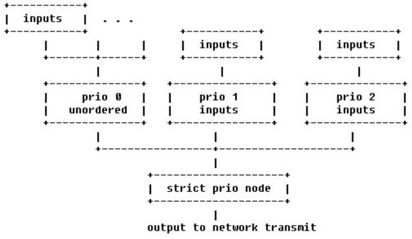
At each node, shaping and dropping parameters may be specified, within limits of the constraints outlined in this document. The following sections detail the device tree attributes applicable for this implementation.
