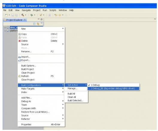
4. **Clean and Build the NIMU driver:** The NIMU driver will be rebuilt in Big Endian format and can now be linked by rebuilt Big Endian NDK examples.
