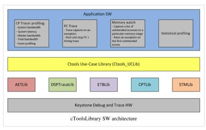
The ctoolslib\_sdk is a collection of libraries for Advanced Triggering(AET), Common Platform Tracers(CPT), Ctools use case library(Ctools UC), DSPTrace, Embedded Trace Buffer(ETB) and System Trace Module(STM) - located \aet\lib. \CPTLib\lib. under \Ctools\_UCLib\lib, \DSPTraceLib\lib, \ETBLib\lib and \STMLib\lib
