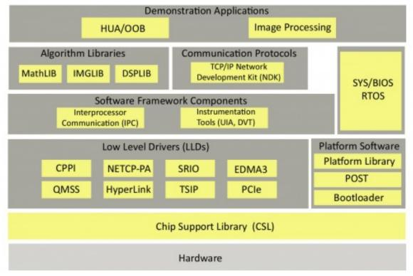
As can be seen in the architecture diagram, the SC-MCSDK consists of those components in the yellow boxes. Specifically they are:
