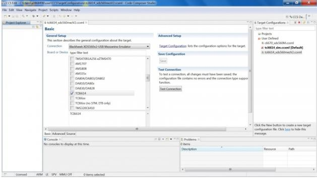
Launch Target configuration for EVM. Click view-> Target Configuration from the top level menu. Inside the Target Configuration window, right click on to the tci6614-evm.ccxml and select "Launch Selected Configuration" as shown below:-
