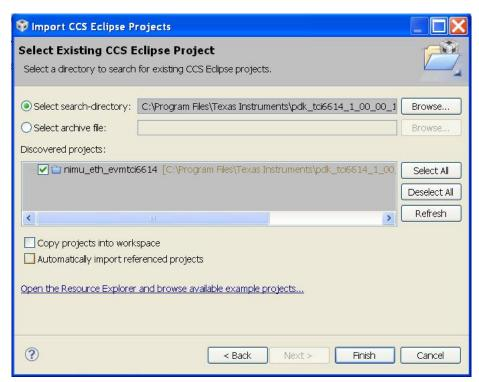
3. Change the NIMU project active build configuration to Big Endian (Debug or Release): In the C/C++ Projects window, right-click on the nimu\_eth\_evmtci6614 RTSC project folder, click on Build Configurations -> Set Active -> Debug\_BE (or Release\_BE for release).
