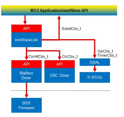
5. 4. 4. 0. 3Figure 26: mmWaveLink - Internal software design
