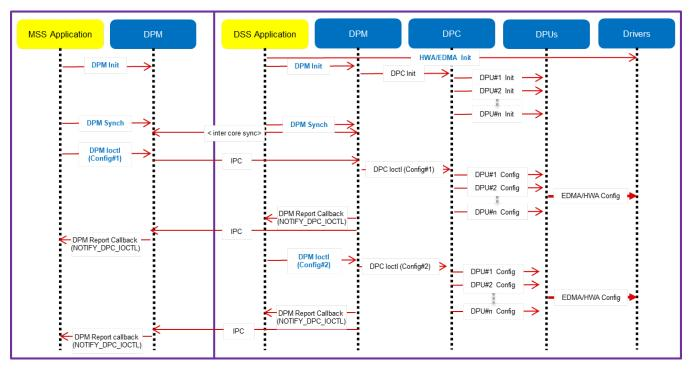
5. 3. 2. 2. 1Figure 21: Data processing flow with remote domain control (init/config)
