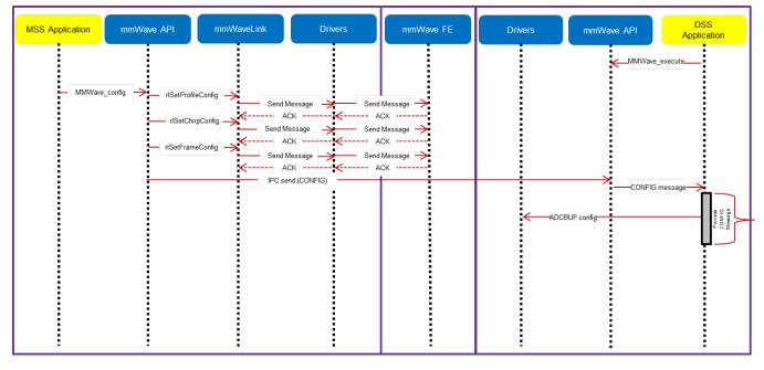
5. 3. 1. 2. 2Figure 16: mmWave Co-operative Mode: Detailed Control Flow (Config sequence)
