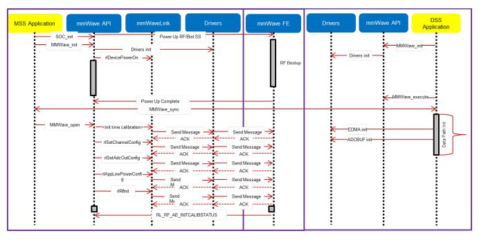
5. 3. 1. 2. 1Figure 15: mmWave Co-operative Mode: Detailed Control Flow (Init sequence)
