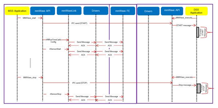
5. 3. 1. 2. 3Figure 17: mmWave Co-operative Mode: Detailed Control Flow (Start sequence)
