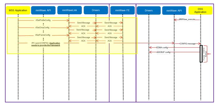
5. 4. 5. 2. 1 Figure 28: mmWave API - 'Minimal' Config - Sample flow (mmWave devices with MSS and DSS cores and module in co-operative mode)
