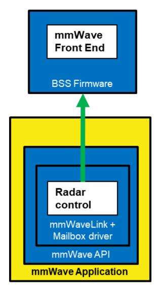
5. 3. 1. 0. 1Figure 11: Typical mmWave radar control flow
