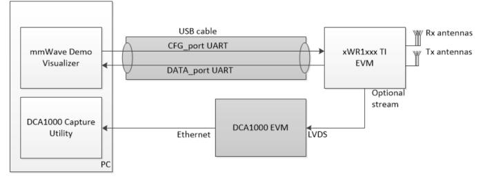
3. 3. 1. 0. 1Figure 1: mmWave Demo Visualizer- mmWave Device Connectivity
