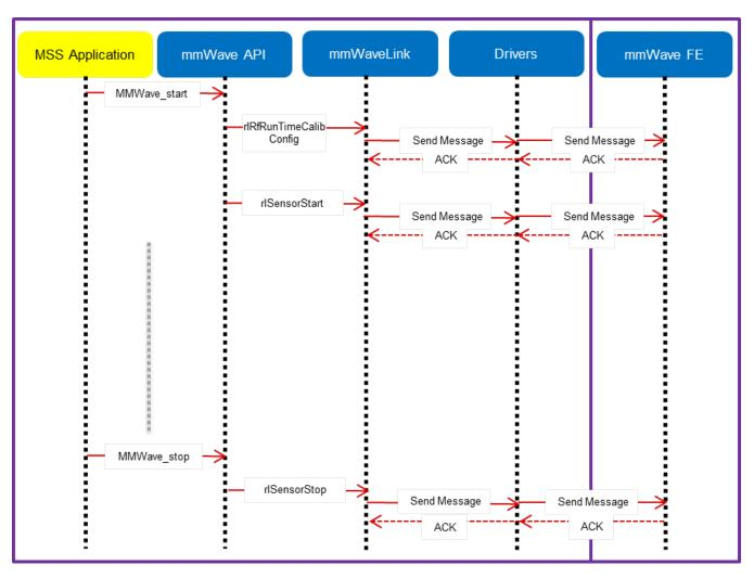
5. 3. 1. 1. 3Figure 14: mmWave Isolation mode: Detailed Control Flow (start sequence)
