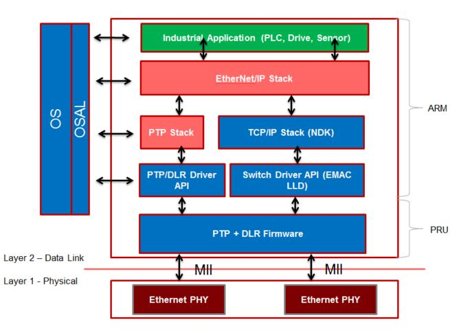
When referring to EtherNet/IP we refer to the layer on top of TCP/IP layer. This can be implemented on the standard switch firmware and does not require any special driver support. The additional features in firmware and driver are PTP and DLR. When referring to the EtherNet/IP driver we refer to the standard switch driver and PTP and DLR driver layers.
