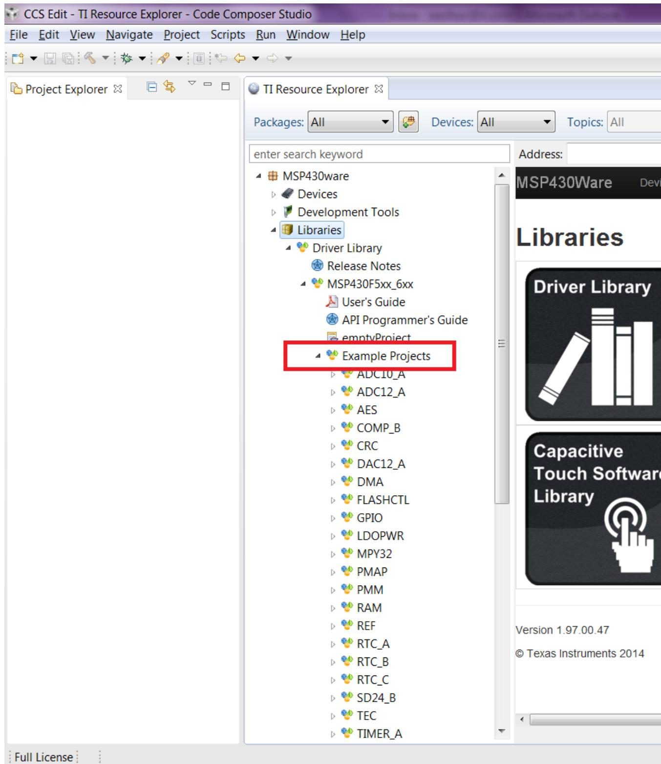
The various peripherals are listed in alphabetical order. The names of peripherals are as in device family user's guide. Clicking on a peripheral name lists the driverlib example code for that peripheral. The screenshot below shows an example when the user clicks on GPIO peripheral.
