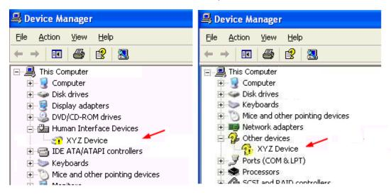
Figure 40. Failed Enumeration Results in the Device Manager
