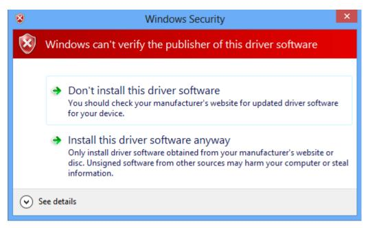
Figure 25. Installing the Driver After Disabling Enforcement
