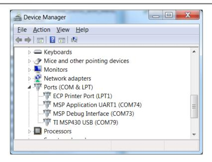
Figure 18. Device Manager with a Fully-Installed CDC Interface
