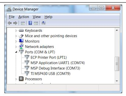
Figure 9. Identifying the COM Port Using the Windows Device Manager
