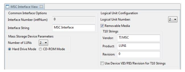
Figure 36. Two-LUN Device; Viewing the Second LUN's Data
