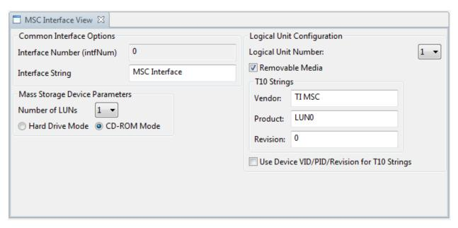
Figure 37. Configuring as a CD-ROM Drive in the Descriptor Tool
