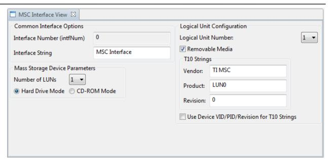
Figure 34. Defining the MSC Interface, in the Descriptor Tool
