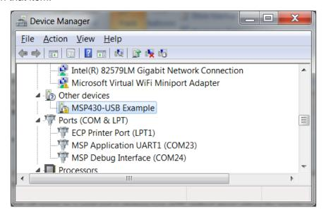
Figure 13. Device Manager Showing CDC Driver Not Installed
