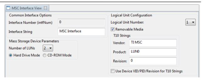
Figure 35. Two-LUN Device; Viewing the First LUN's Data
