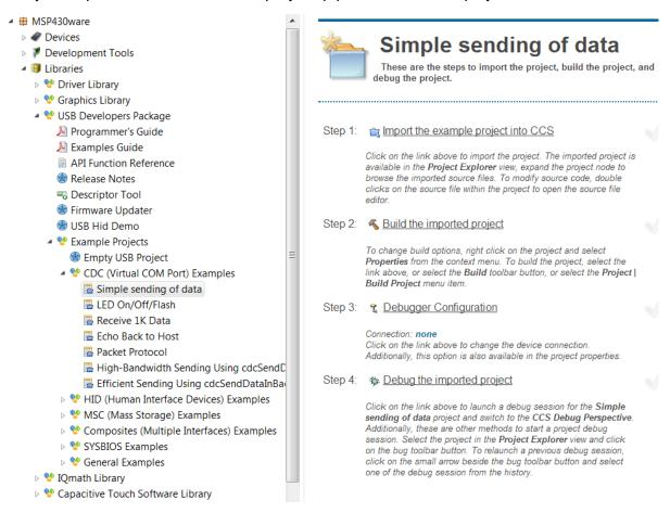
Figure 1. Viewing the Examples in the TI Resource Explorer
