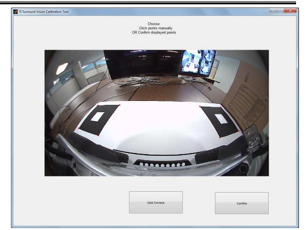
Figure 13: Step 4.3 – Confirmation of clicked points. If un-satisfied with clicked points for the image use the button "click corners" and redo corner selection
