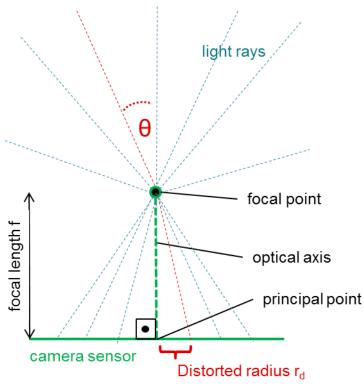
Figure 8: Camera with Lens Distortion
