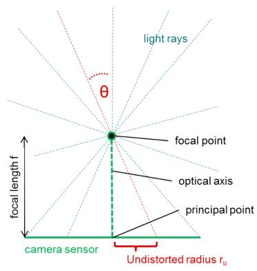
Figure 7: Pinhole Camera (distortion-free)
