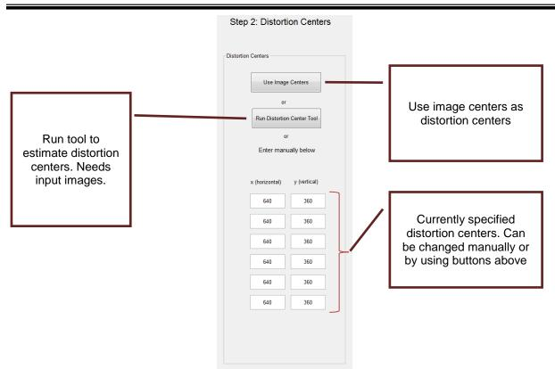
Figure 4: Step 2 - Distortion Centers
