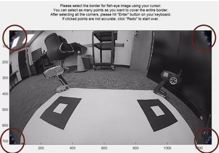
Figure 5: Distortion Center Tool
