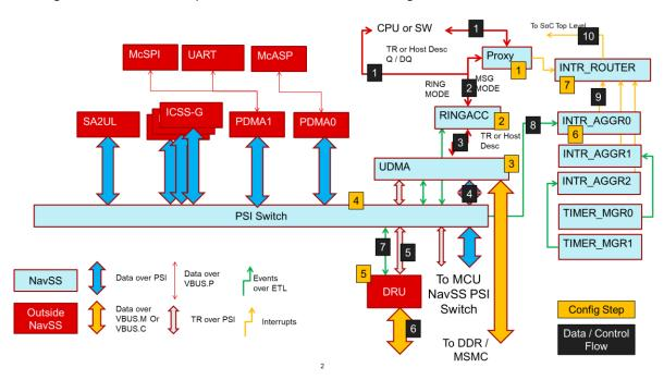
Figure 4. AM6x Main NavSS: SW view and DRU UDMA sequence
