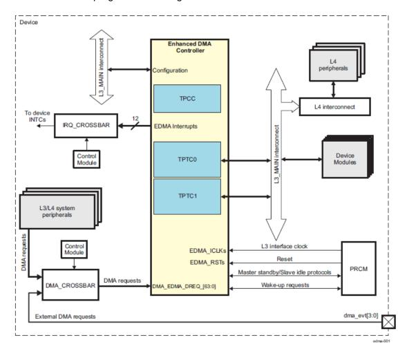
Figure 1. EDMA in AM5x SoC
