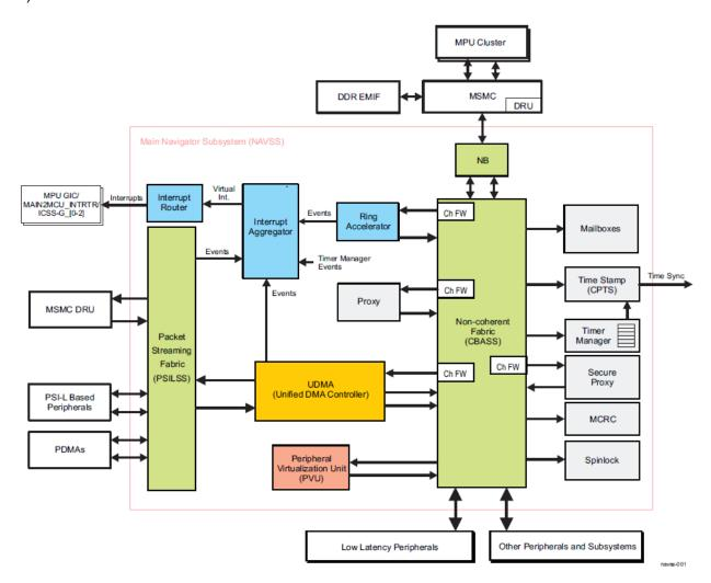
Figure 2. Main NavSS Block Diagram in AM6x SoC
