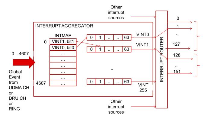
Figure 9. AM6x SoC Main NavSS UDMA Interrupt Aggregator and Interrupt Router
