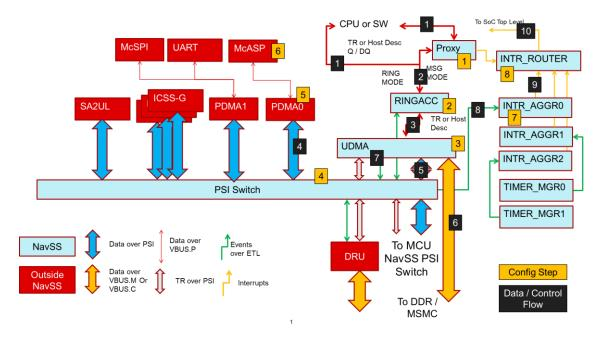
Figure 3. AM6x Main NavSS: SW view and McASP UDMA sequence
