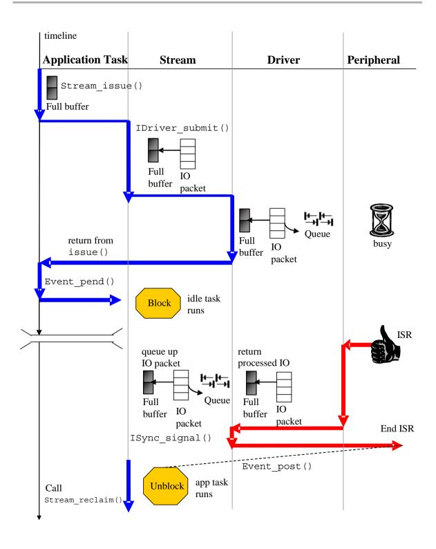
The following example uses Stream\_issue() and Stream\_reclaim() with an Event. "Generator" is a driver provided with SYS/BIOS. The Event and the Generator driver are statically created in this example. This example uses the genSine and myPrintf functions from the previous section; they are not repeated in this example.
