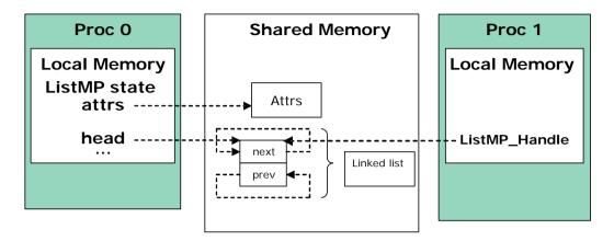
The cache alignment used by the list is taken from the SharedRegion on a per-region basis. The alignment must be the same across all processors and should be the worst-case cache line boundary.
