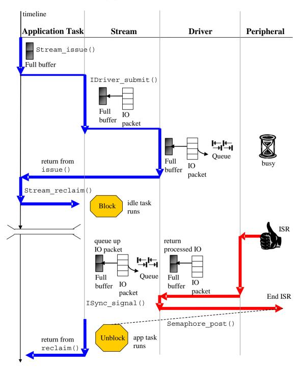
The following example uses Stream\_issue() and Stream\_reclaim() in a Task. "Generator" is a driver provided with SYS/BIOS. All instances are dynamically created in this example.
