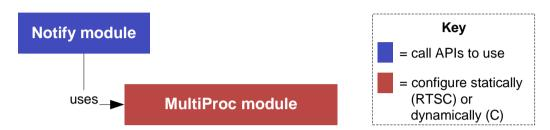
In this scenario, you make API calls to the Notify module. For example, the Notify\_sendEvent() function sends an event to the specified processor. You can dynamically register callback functions with the Notify module to handle such events.
