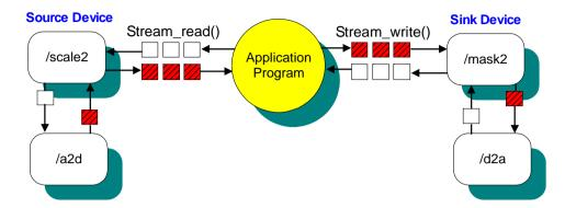
Stacking drivers do not implement the IDriver interface. Instead, they implement a different interface called IConverter. Converters are not added to the driver table. Instead, the Stream module maintains a table of converters. Stream searches both the converter table and the driver table for matches. However, note that names must be unique within all the items in both tables. The Stream module searches the converter table first.
