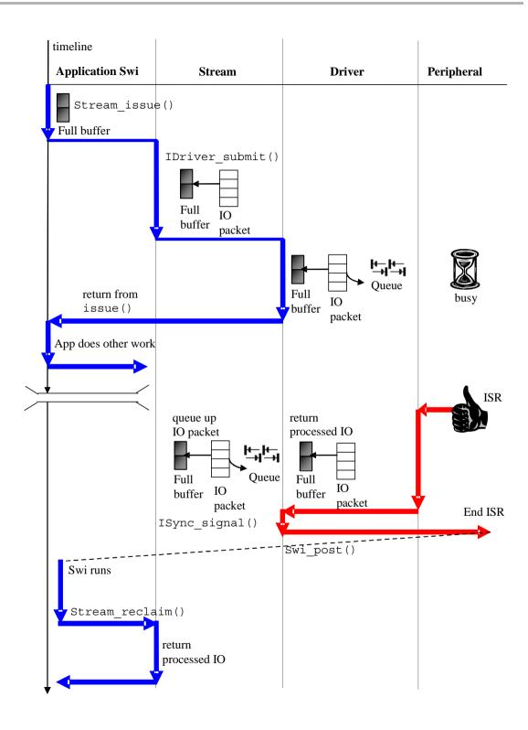
The following example uses Stream\_issue() and Stream\_reclaim() in a Swi. "Generator" is a driver provided with SYS/BIOS. All instances are statically created in this example. This example uses the genSine and myPrintf functions from the previous section; they are not repeated in this example.
