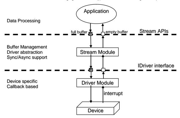
In this use case, the application calls Stream module APIs. Those APIs manage buffers and the driver abstraction. Internally, the Stream module APIs calls the implementation of the IDriver interface for the driver.
