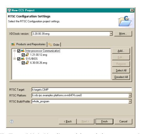
NOTE: The available build profiles are **debug**, **whole\_program**, and **whole\_program\_debug**. The default is whole\_program. The "debug" profile allows you to step through the sources if sources are available. The "whole\_program" profile has negligible debug symbols. The "whole\_program\_debug" profile has more debug symbols and improves the debug experience when compared to "whole\_program". It is recommended that production code be built with whole\_program or whole\_program\_debug.
