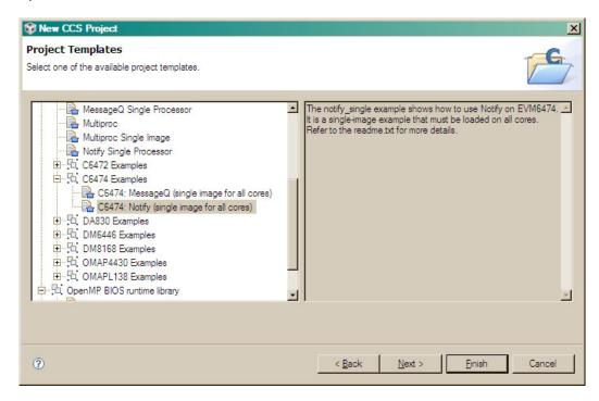
7. Ensure that the correct repositories are selected and then select the IPC platform corresponding to your device/core. I.e. for c6474:
