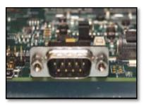
Connect the provided RS-232 null modem cable to the EVM UART port. The other end of the cable needs to be connected to your Linux development host.
