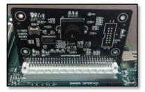
Connect Sensor module to main board
