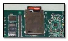
Insert the SD card containing the Linux demo image into the SD/MMC slot
