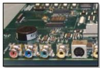
Connect your 1080p display to the component video out RCA connector. Power on the HD video display.
