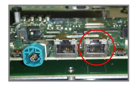
5 Connect the Ethernet cable to the port P5 on the board. Connect the other end of the cable to an Internet-ready connection
