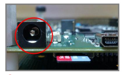
6 Connect the supplied 12-V (7A) DC power supply to the EVM (J3).
