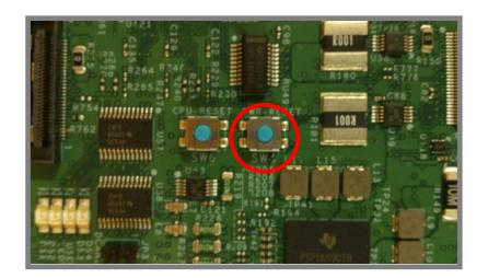
Press the Power On button (SW4) to boot the board with the SD card.
