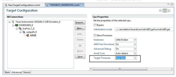
Note that the XDS100v2 users should upgrade to the latest CPLD. An upgrade of the CPLD will improve reliability for adaptive clocking connections. To update the XDS100v2 CPLD, please see XDS100#Q: How\_can\_I\_update\_the\_CPLD\_on\_my\_XDS100v2.3F
