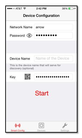
The SmartConfig operation should complete in a few seconds. However, the operation can take up to two minutes to complete. The red LED should go off once connected.
