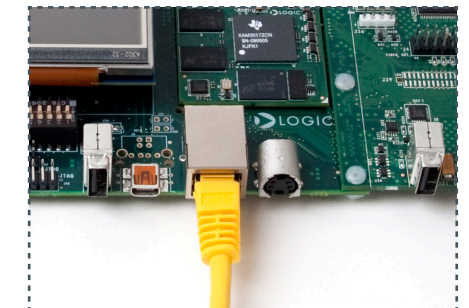
6 Connect Ethernet cable to baseboard and Internet-ready connection, such as a network router
