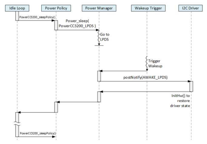
The power policy calls the Power\_sleep() API to activate the power savings. The processor stays in the sleep state until a wakeup event occurs. The available wakeups vary by device and sleep state, but in general the processor wakes up due to a timed wakeup (from a timer active during the sleep state) or an interrupt signal from an external input, or from a network coprocessor.
