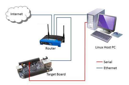
5. Use the SD Card to boot the target boardproperly connected for your development environment
