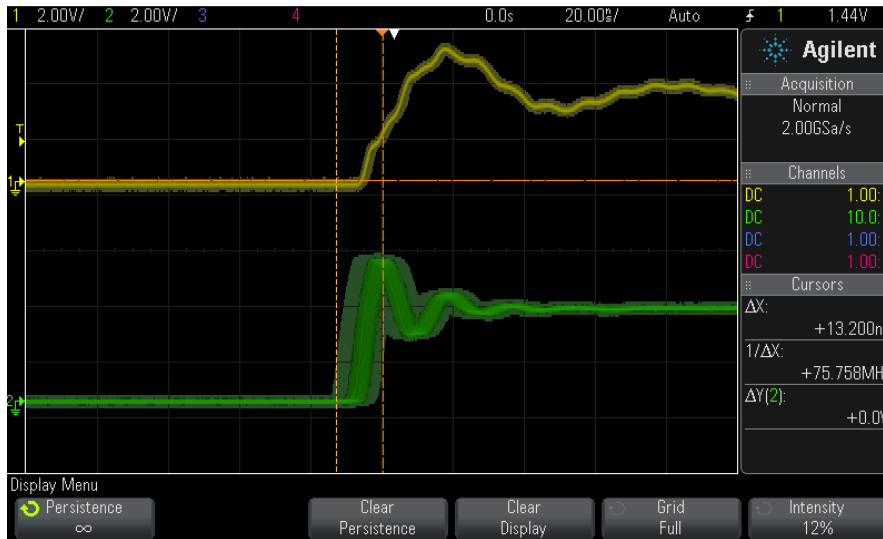
Topology (1) oscilloscope capture showing Sync Pulse jitter measurement between two AM335x ICE boards
