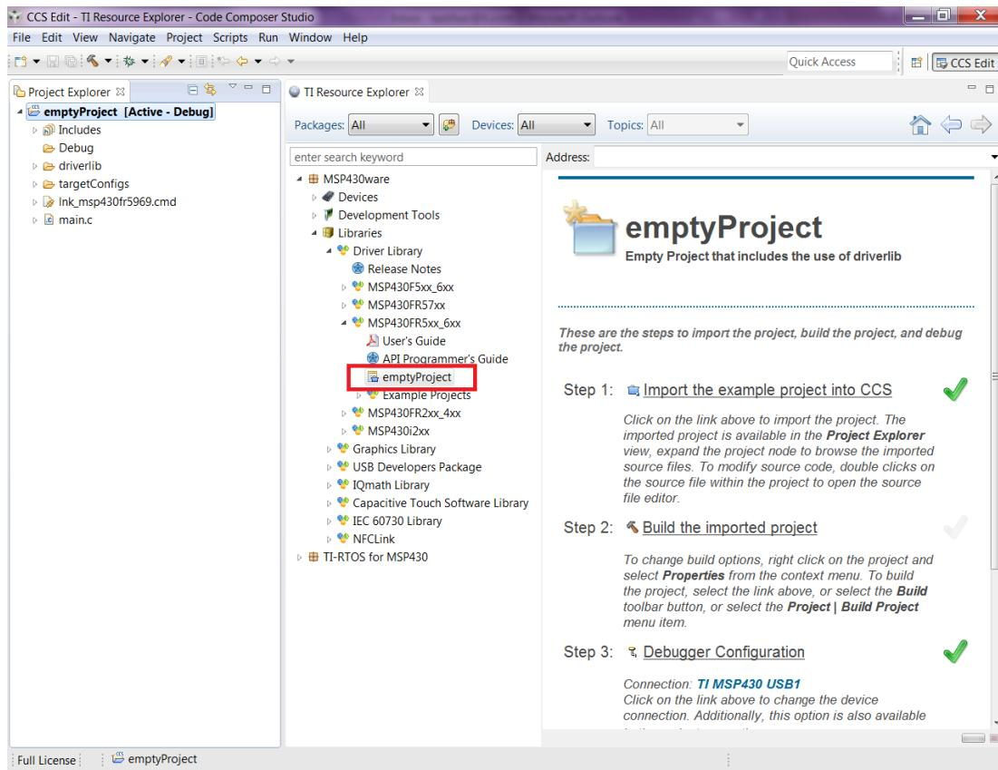
The `main.c` included with the empty project can be modified to include user code.
