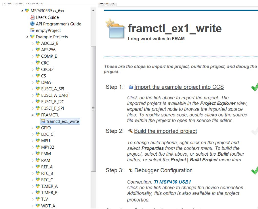
The imported project can be viewed on the left in the Project Explorer. All required driverlib source and header files are included inside the driverlib folder. All driverlib source and header files are linked to the example projects. So if the user modifies any of these source or header files, the original copy of the installed MSP430ware driverlib source and header files get modified.
