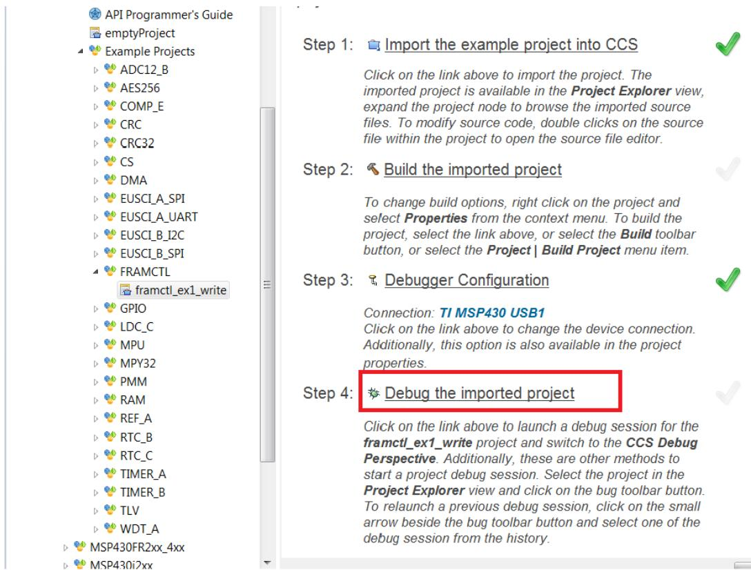
The COM port to download to can be changed using the Debugger Configuration option on the right if required.
