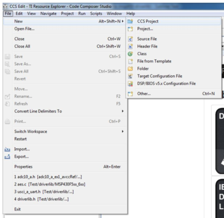
Once the new project wizard has been opened name your project and choose the device you would like to create a Driver Library project for. The device must be supported by driver library. Then under "Project templates and examples" choose "Empty Project with DriverLib Source" as seen below.
