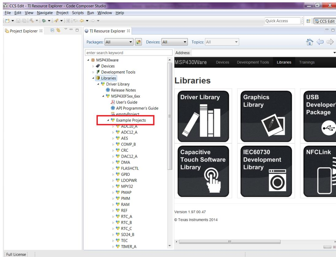
The various peripherals are listed in alphabetical order. The names of peripherals are as in device family user's guide. Clicking on a peripheral name lists the driverlib example code for that peripheral. The screenshot below shows an example when the user clicks on GPIO peripheral.
