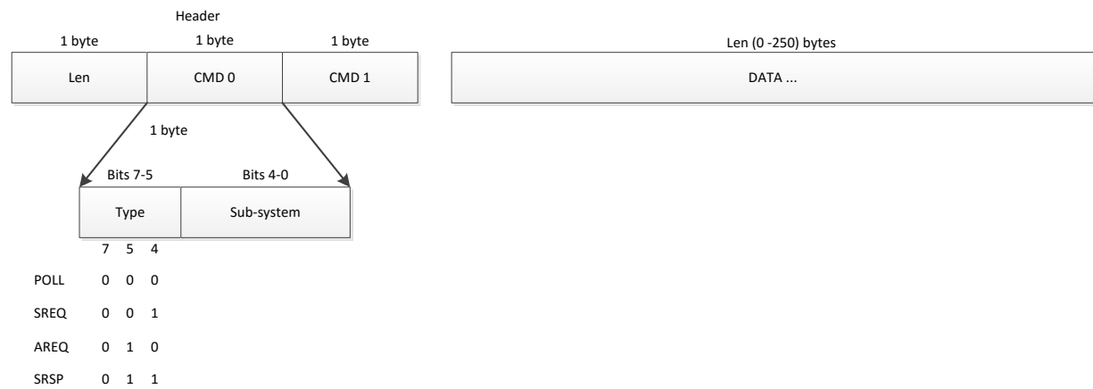
Figure 5: Standard MT Frame Format
