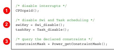
The next step determines whether the constraints prevent the use of the Deep Sleep 1 state, the deepest level (step 4). If this state is allowed, Power\_sleep() is called (step 5). When the device returns from Deep Sleep 1, a flag is set to indicate that the device slept (step 6).
