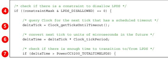
If there is sufficient time to transition in and out of LPDS, then the policy has come to the decision to enter LPDS. However, there will be some latency to wake up the device from LPDS to be ready to perform the processing that is scheduled. To ensure that the processor is ready in time to perform the scheduled processing, the policy needs to compute an earlier wakeup time to accommodate the wake latency (later, in step 12).
