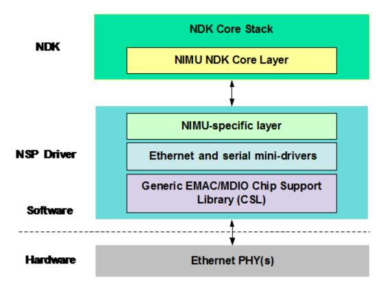
This new NSP Ethernet driver architecture consists of the following components:
