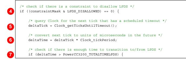
If there is sufficient time to transition in and out of LPDS, then the policy has come to the decision to enter LPDS. However, there will be some latency to wake up the device from LPDS to be ready to perform the processing that is scheduled. To ensure that the processor is ready in time to perform the scheduled processing, the policy needs to compute an earlier wakeup time to accommodate the wake latency.
