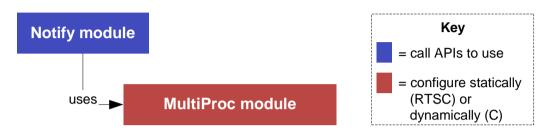
In this scenario, you make API calls to the Notify module. For example, the Notify\_sendEvent() function sends an event to the specified processor. You can register callback functions with the Notify module to handle such events either statically or dynamically.
