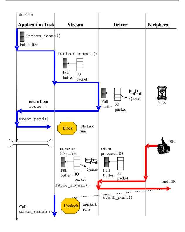
The following example uses Stream\_issue() and Stream\_reclaim() with an Event. "Generator" is a driver provided with SYS/BIOS. The Event and the Generator driver are statically created in this example. This example uses the genSine and myPrintf functions from the previous section; they are not repeated in this example.
