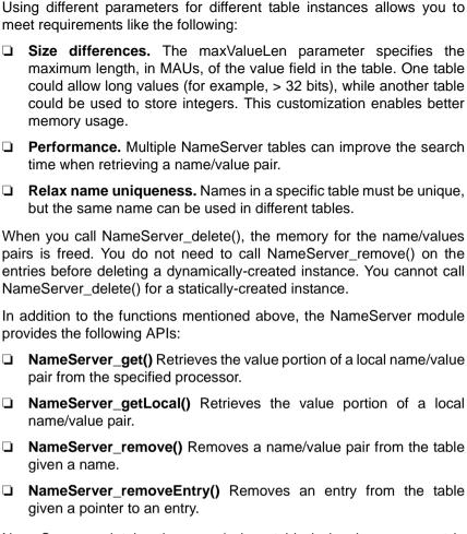
NameServer maintains the name/values table in local memory, not in shared memory. However the NameServer module can be used in a multiprocessor system. The module communicates with other processors via NameServer Remote drivers, which are implementations of the INameServerRemote interface. The communication to the other processors is dependent on the Remote drivers implementation. When a remote driver is created, it registers with NameServer via the NameServer\_registerRemoteDriver() API.
