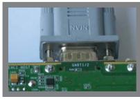
Connect the supplied serial cable to the UART-1/2 DB-9 connector. Connect the other end of the cable to a PC or workstation.
