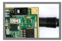
Connect the power cable to the power jack on the main board. It is recommended to complete this step before connecting the power source. As there is no power switch on the EVM, use the cord for power cycling the board.
