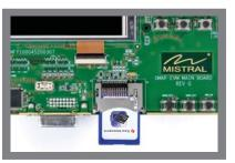
Insert the Linux SDK SD card into the AM/DM37x
