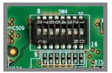
Ensure SW4 DIP switch is set as shown. SW4 DIP is located on the front of the AM/DM37x EVM main board.
