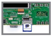
Insert the Linux SDK SD card into the OMAP35x EVM as shown.
