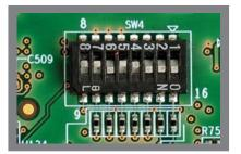
Ensure SW4 DIP switch is set as shown. SW4 DIP is located on the front of the OMAP35x EVM main board.
