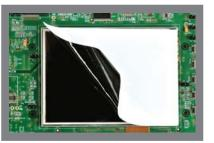
Remove the protective plastic from the LCD touchscreen.
