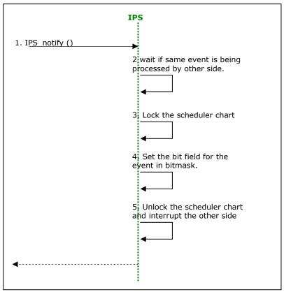
Figure 6. On the GPP: IPS\_notify() control flow
