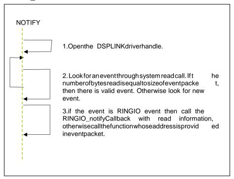
Figure 10. On the GPP: NOTIFY\_eventWorker() control flow
