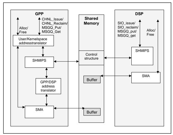
Figure 3. ZCPY sub-component interaction
