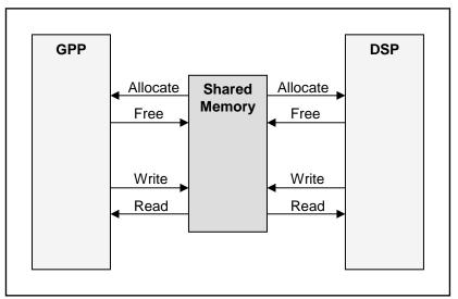
Figure1. BasicarchitectureofsystemsupportingZCPYtransf ermode
