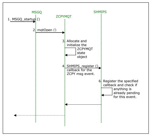
Figure 10. On the DSP: ZCPYMQT\_open() control flow
