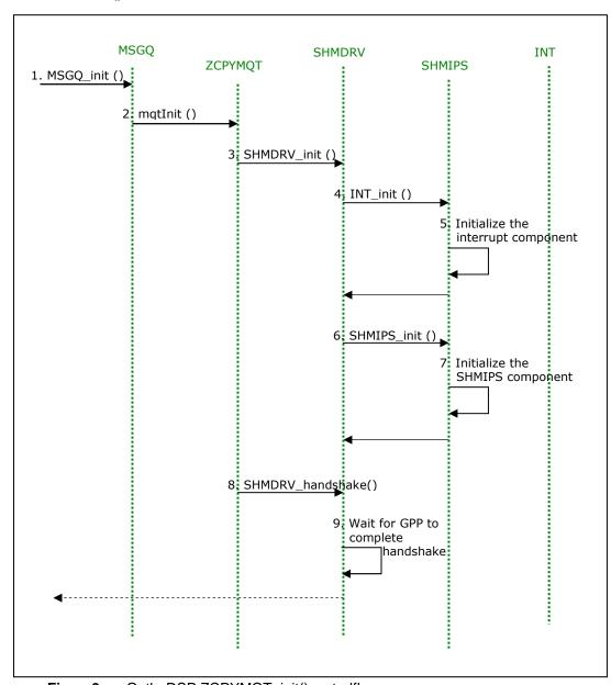
Figure 9. On the DSP: ZCPYMQT\_init() control flow
