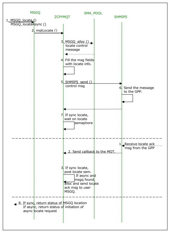
Figure 13. On the DSP: ZCPYMQT\_locate() control flow
